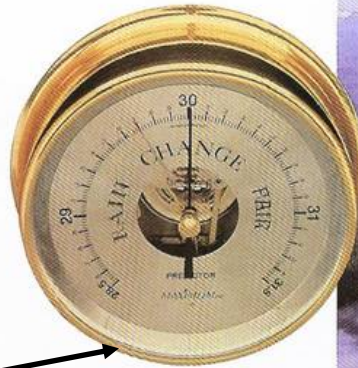
Figure 3-26 An aneroid barometer (inset) is used to measure air pressure anywhere from your hometown to the foggy banks off Kruzof Island in Alaska.
